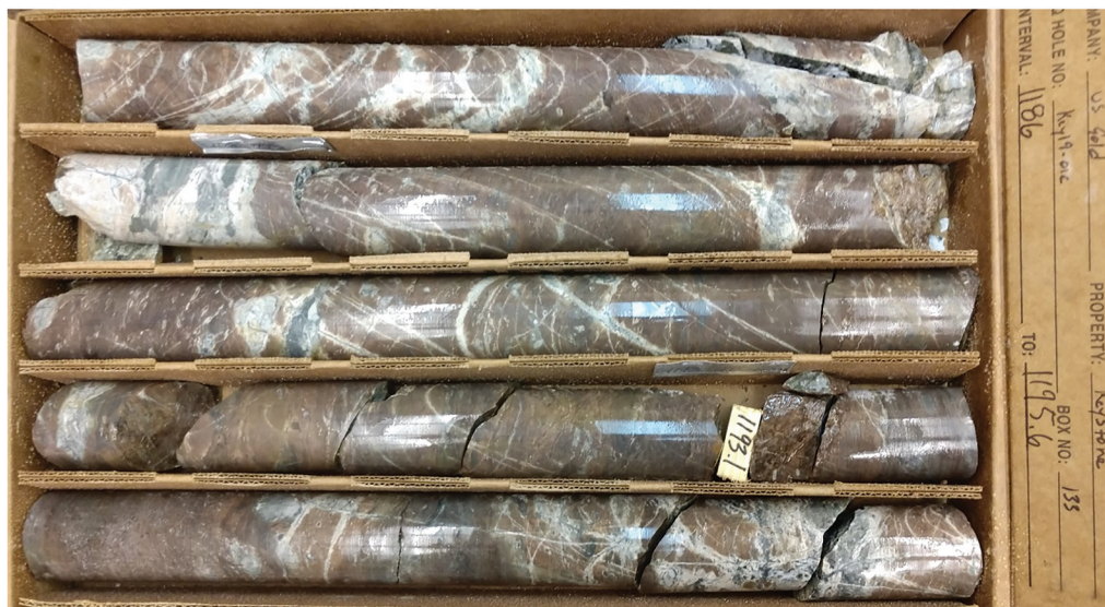
Figure 14. Lower Comus hornfels, “biotite hornfels”, cut by fracture-controlled skarn of currently uncertain mineralogy. Interval assayed 10–32 ppb Au with anomalous Cu-Bi-Te-Tl.
