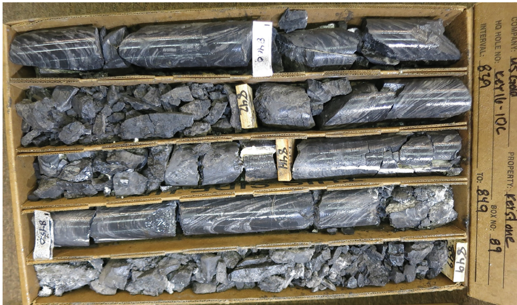
Figure 7. Cambrian-Ordovician Comus Formation limestone and calcareous siltstone. Note tight folding and rhythmic bedding of silty versus muddy beds, very favorable characteristics for Carlin-style alteration and gold deposition.
