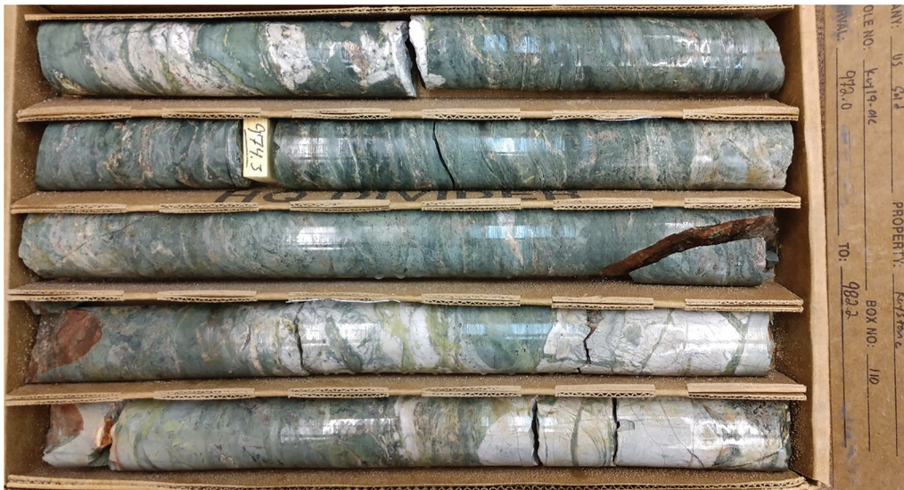
Figure 15. Comus garnet-pyroxene skarn with retrograde quartz-chlorite-epidote-pyrite alteration. Lighter colored rock at lower right is greenstone. Interval assayed 42–119 ppb Au with anomalous Ag-Bi-Te.
