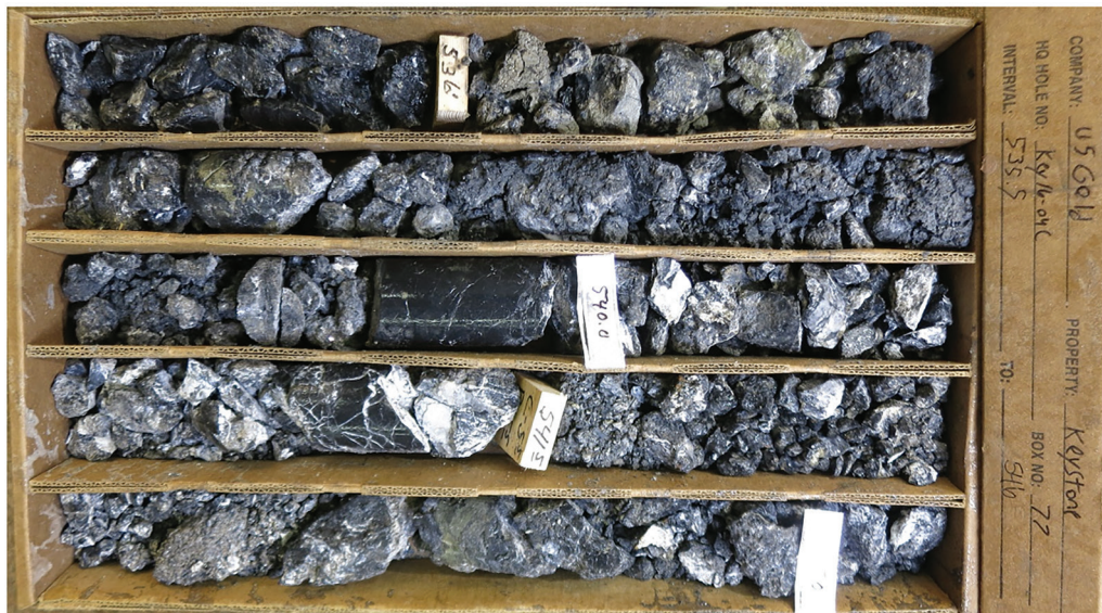
Figure 19. Jasperoid developed in Wenban limestone directly below the Roberts Mountains Thrust. Interval assayed < 5 ppb Au with anomalous As-Hg-Sb-Tl-Zn.
