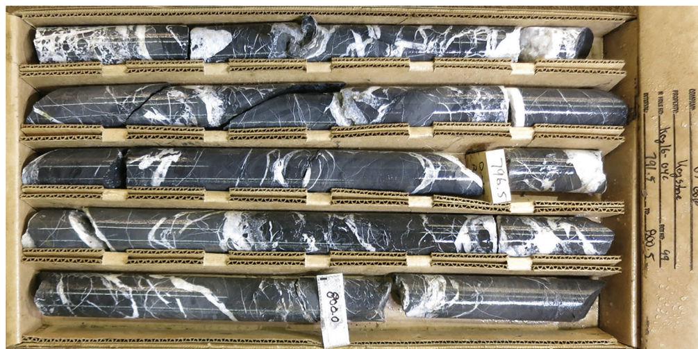
Figure 20. Calcite veinlet swarm (“Calcite Halo”) below jasperoid developed in Wenban limestone. Interval assayed < 5 ppb Au with weakly anomalous Ba and Sb.
